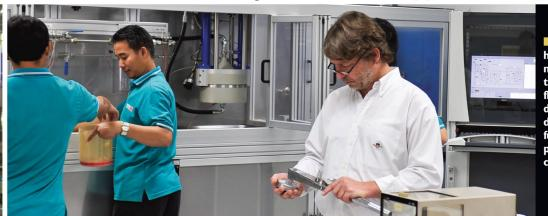
Hiflofiltro uses high-tech laser technology to measure the filtering efficiency, flow and pressure drop, helping them to design filters that will function with optimal performance under all circumstances.
